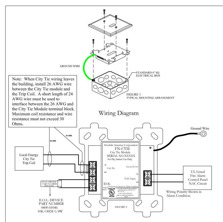
All Wiring is Power Limited, Connect only to Power Limited Circuits. For Use Only With Supervised Circuits.
